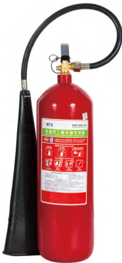
MT/5 CO 2 FIRE EXTINGUISHER 5kg Diameter: 155mm Maximum working pressure: 17Mpa Test pressure: 25Mpa Minimum wall thickness: \geq 3.0\text{mm} Material: Steel Fire Rating: 34B Standard: CCS / ZY / EC
