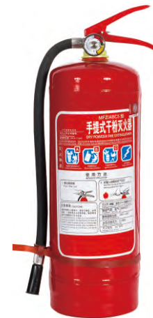
MFZ/ABC 5kg POWDER FIRE EXTINGUISHER Diameter: 150mm Maximum working pressure: 1.2Mpa Ambient temperature: -20^{\circ}\text{C} \sim +55^{\circ}\text{C} Test pressure: 2.1Mpa Minimum wall thickness: \geq 1.3\text{mm} Material: Carbon Steel Fire Rating: 3A89B Standard: CCS / ZY / EC
