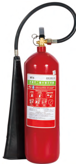
MT/7 CO 2 FIRE EXTINGUISHER 7kg Diameter: 155mm Maximum working pressure: 17Mpa Test pressure: 25Mpa Minimum wall thickness: \geq 3.4\text{mm} Material: Alloy Steel Fire Rating: 55B Standard: CCS / ZY / EC
